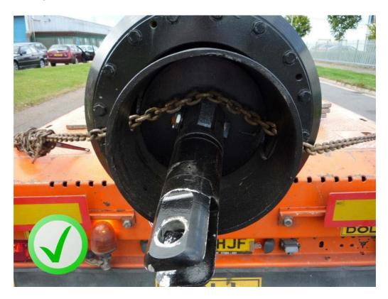
In general, the Kelly bar should travel with the swivel fitted but if it has been removed for some reason this can create a potentially dangerous situation during transportation – in many cases the swivel also acts as a retainer for other heavy components so if it has been removed the other components may fall from the truck during transport. If the swivel is not present please discuss the implications of this with your supplier prior to organising transport.
