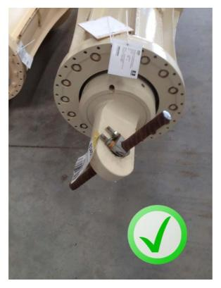
In the absence of a swivel a temporary locking bar can be fitted as shown to the left here. This arrangement prevents the bar from extending during transportation or handling.
