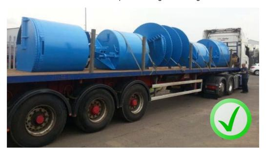
Where buckets are loaded on their sides, and they are fully circular, they are likely to roll around on the truck bed so they must be chocked in such a way as to
