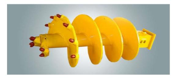
There are different types and designs of augers but in general these items are circular in design with varying diameters and lengths. Prior to loading the site must check that all wear parts are secure. If they are loose, they should be removed and handed to the truck driver for safe storage and a comment about that added to the collection/delivery note. Failure to do so may result in a dangerous occurrence during loading/off-loading or an item falling from the truck during transit.
