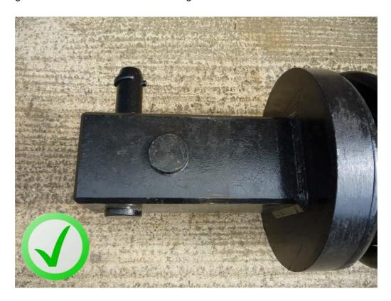
The Kelly swivel (top end of the bar) must also be checked for security prior to loading.
