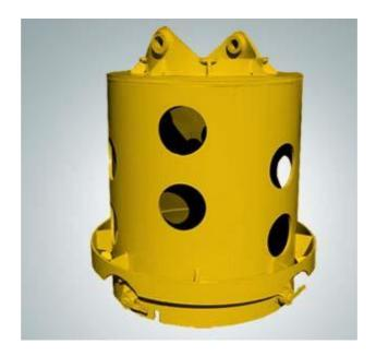
Casing Drive Adapters typically contain locking pins. These locking pins must be checked for security prior to loading on a truck. If they are loose, they should be removed and handed to the truck driver for safe storage and a comment about that added to the collection/delivery note.
