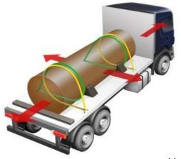
Where shorter casings are loaded on their end it is important to determine that they will remain stable during transit. It is good practise to load the casings onto packing timbers (in order to spread the load and protect the truck bed but also to assist in their off-loading at the return address). Make sure to use sufficiently large sections of timber and of sufficient length/strength when doing this, creating a level, stable and sufficiently wide temporary platform
