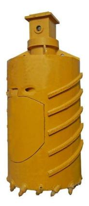
There are different types and designs of buckets but in general these items are circular in design with varying diameters and lengths. They typically contain swinging or hinged doors and may have automatic or manual release mechanisms. With more moving parts they are perhaps more susceptible to being damaged in use than some other tools and this may have a more significant effect on loading and transport planning.
