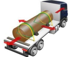
significant overhang or gap between supports may lead to a permanent bend in the auger and any repair/replacement associated with this outcome will result in a cost to the job site. [Picture required]
