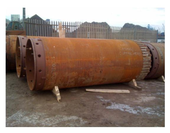
These twin wall casings can be supplied in a wide range of standard diameters and in various lengths typically from 1.0m up to 6.0m, each with a known weight. They typically contain a number of casing screws which are threaded radially into on end of the casing. Some lengths of casing may also contain cutting teeth and these can be welded or removable.
