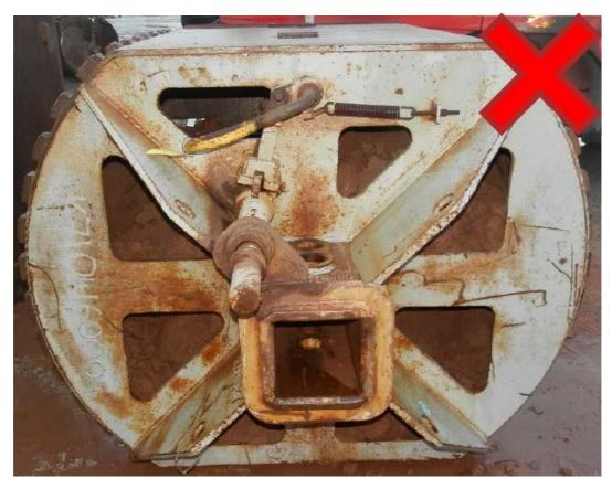
Prior to loading the site must check that all mechanisms and potentially loose wear parts are secure. Failure to do so may result in a dangerous occurrence during loading/off-loading or perhaps result in an item falling from the truck during transit. If they are loose, they should be removed and handed to the truck driver for safe storage and a comment about that added to the collection/delivery note.
