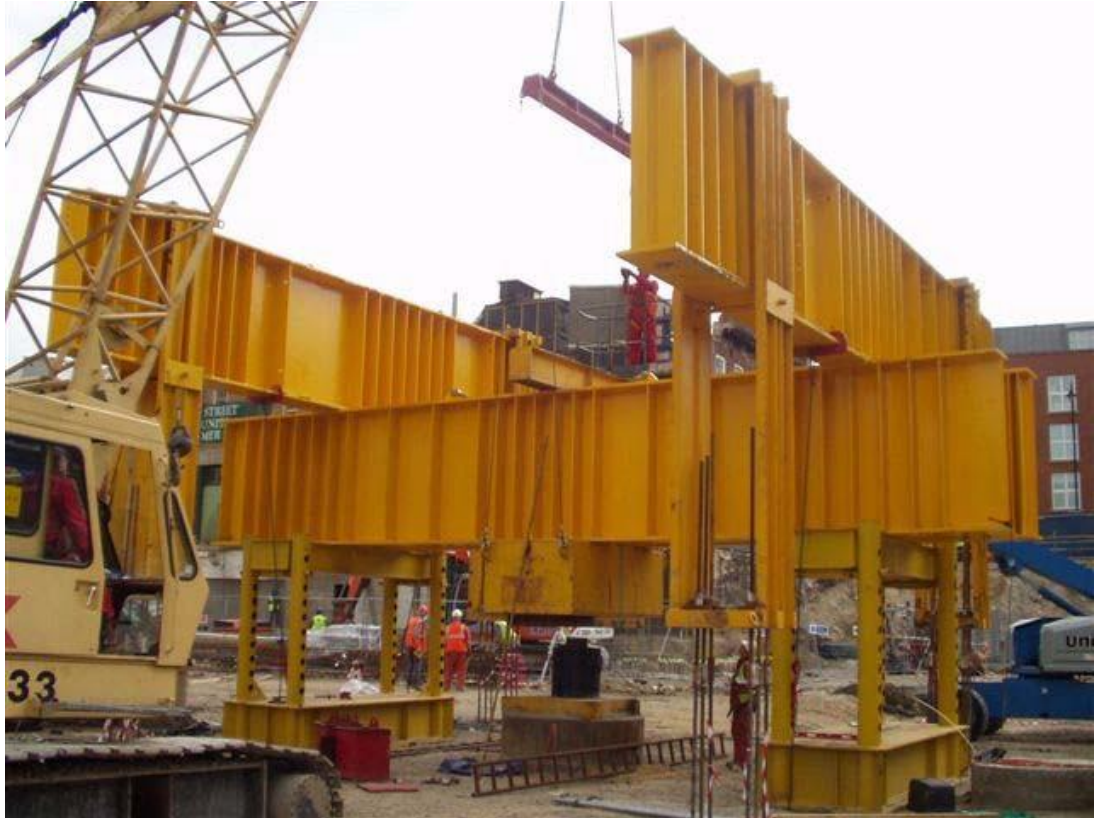
Figure 5.1 30MN reaction pile test
