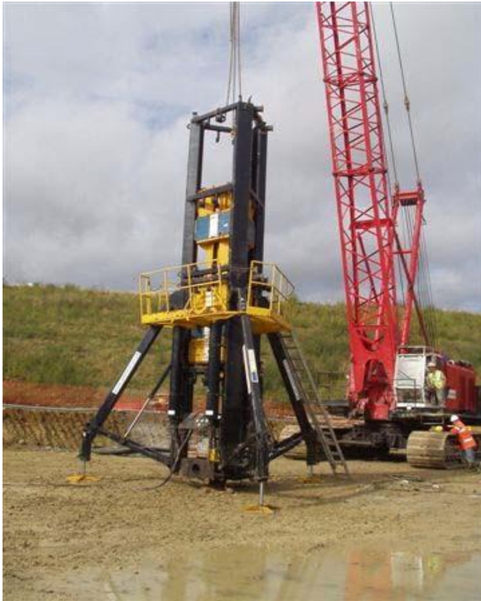
Figure 5.7 3MN capacity test
