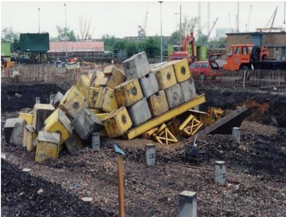
Figure 2.2 Platform bearing failure under kentledge test
