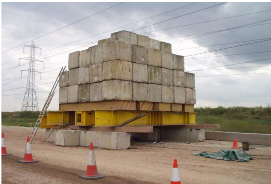
Figure 5.3 3MN kentledge test
