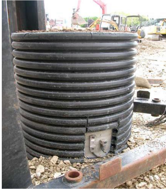
Figure 5.10 Bored cast in place/CFA pile head preparation with window cut in liner to allow strain gauge and accelerometer to be attached to the pile
