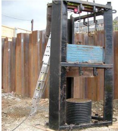
Figure 5.9 Dynamic load testing of cast-in-place pile
