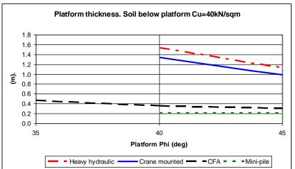
For further details refer to BRE Report 470, Working Platforms for Tracked Plant: good practice guide to the design, installation, maintenance and repair of ground-supported working platforms.
