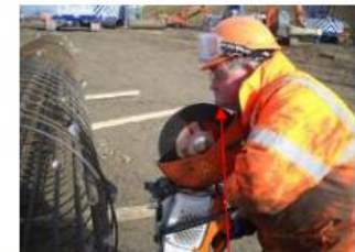
Position of tool and blade after kickback
