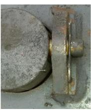
Hi Tensile bolt and nylok nut fitted after event.
