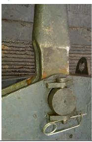
Different size / strength 'nappy pins' used on the hammer/ mast guides.
