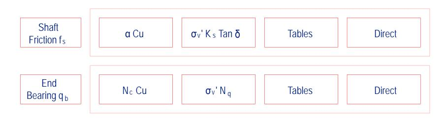
The similarity is that all methods end up with f<sub>s</sub> and q<sub>b</sub>, whether this is the German EA-Pfähle, UK φ' and Cu methods, the French PMT methods or other methods in use elsewhere in Europe
