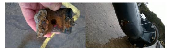
A recent incident occurred during a lifting operation involving a 9mtr auger extension being lifted into the rotary table on an Soilmec SR95. A lifting bracket became detached from the swan neck. This was the result of a defective weld created by the manufacturer. In this instance there were no injuries to any personnel.
