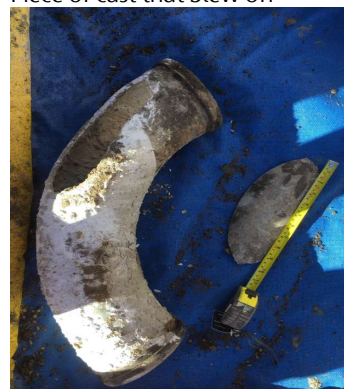
Piece of cast that blew off
