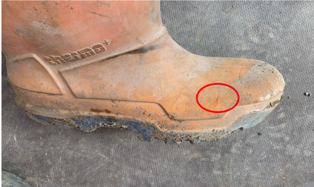
Damage sustained to the IP's boot from the jet wash.
