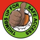
Red Zone: The Rig Operator must ensure the rig is placed in a safe condition before an Authorised Person enters the Red Zone. The operator must give a 'Thumbs up' to the Authorised Person wanting access confirming it is safe to enter before they enter the Red Zone.
